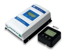
MPPT solar controllers (maximum power point tracking) are needed as a link between the solar panels and the batteries. With the MPP technology, the controller automatically determines the maximum power output of the solar panels at all times. This reduces the charging time of the battery significantly compared with the conventional solar chargers. The MPPT solar controllers work fully automatically, with a charging current of up to 30A or 40A and they are maintenance free.
